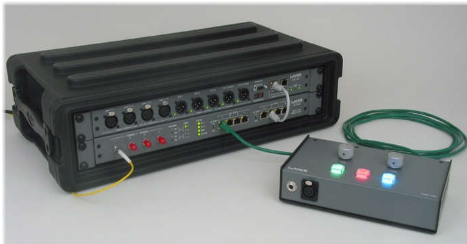
Typical booth system with the ADX-8000 switch/power supply and an ADX-140 XLR Interface unit.
